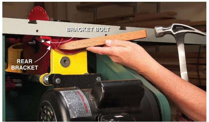
Shift the rear trunnion bracket by slightly loosening its bolts and gently tapping left or right with a hammer and a pointed stick. The blade moves with the bracket. This crude method works OK, but you'll find installing a PALS system makes this adjustment much easier.
