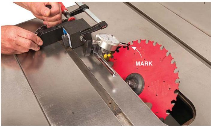
Measure the blade's alignment at 45°. Repeat the same front-and-back measuring procedure you used to align the blade at 90°. This time, the blade is tilted away from the dial indicator.
